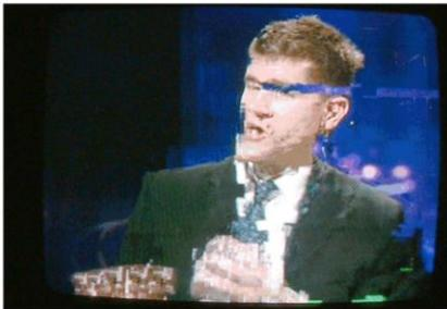
Fig 4.2.2. The result of severe DTT signal degradation is 'pavilion' and a stop-start picture.
