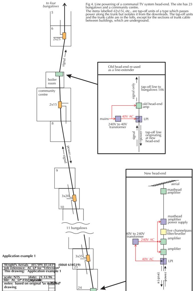
Fig.4: Line powering of a communal system head-end
