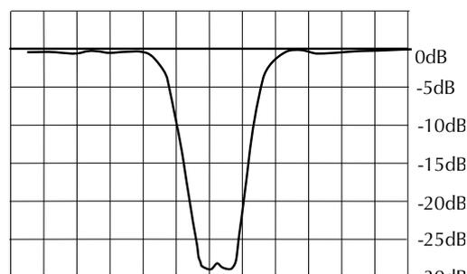
Fig. 5. Frequency response of a double notch filter, with the tuning staggered slightly. A deeper and narrower notch is obtained if the two stages are tuned to precisely the same frequency.
