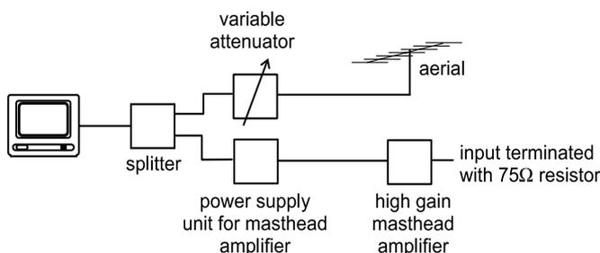
Fig. 2. Test set-up to show that lifting the noise floor has the same effect on the picture as reducing the signal level
