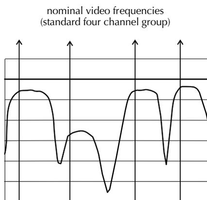
Fig. 4. Frequency response of a four channel pass filter. One channel has been set at -10dB
